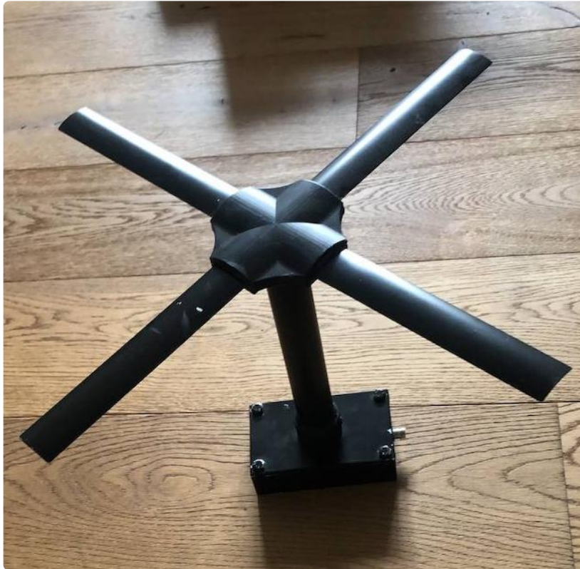
Figure 1: Assembly Model 1 with base plate, enclosure with socket, Ø32 mm tube, and head_v2 with aluminum strip elements.
